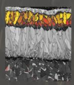
Conventional CVD alumina coating with random crystal orientation.
