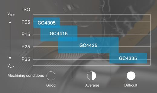
First-choice grade GC4425 delivers improved wear resistance, heat resistance and toughness, significantly expanding the application range.
