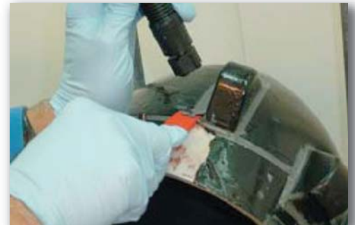
Edge Sealant Removal
