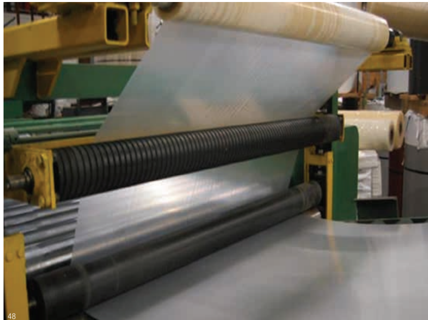
To help ensure a scratch-free surface for the end user, 3M™ Co-Extruded “A” Tape is applied after final finishing to sinks, spas, and countertops prior to packaging. Enhanced abrasion and puncture resistance protects the surface through shipping and installation. Tape then removes cleanly.
