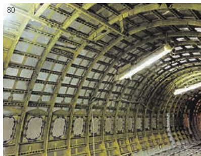
3M™ Damping Foil 435 between the ribs and stringers of an aircraft fuselage helps reduce vibrational fatigue and noise inside the passenger cabin.
