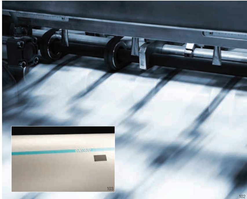
3M™ Repulpable Splittable Flying Splice Tape eliminates the time and work of “V” and “W” patterns with a straight across flying splice. Advanced coating provides a smooth and consistent opening force. A fiber-free break open means less blanket cleanup.
