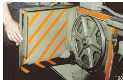
Orange 3M™ Vinyl Tape identifies dangerous machine parts that may cause injury when enclosure doors are open or guards removed.
