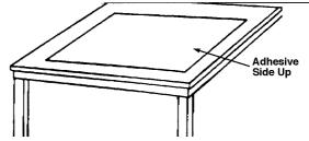
Align the graphic face - down on the application tape adhesive. See FIGURE 3.
