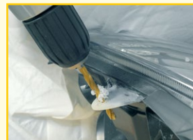
Shape and drill the repaired part within just a few minutes and paint as required
