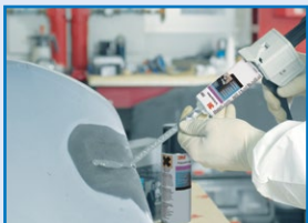
Fill the crack with FPRM plastic repair material to create a smooth, flexible, long lasting surface to paint
