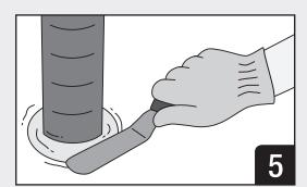
Tool sealant to be flush with substrate.
