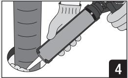
Apply sealant to required depth in annular space per system specifications. Completely fill annular space with sealant.
