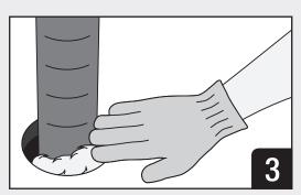
When applicable, install mineral wool to required depth per system specifications.
