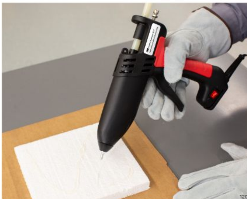
3M™ Hot Melt Applicator LT with 3M™ Hot Melt Adhesive 3782LM low temperature (265°F/129°C) adhesive effectively bonds heat-sensitive substrates such as styrene foam to itself, corrugated or other surfaces without damaging the foam.
