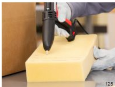
3M™ Hot Melt Applicator LT and 3M™ Hot Melt Adhesive 3782LM applied at low temperature (265°F/129°C) make quick work of wetting, gimping, and bonding fabric to wood.
