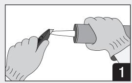
Cartridge: Cut off tip of nozzle to desired size.
