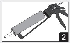
Cartridge: Insert cartridge into cartridge applicator.
