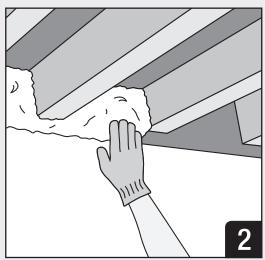
Install mineral wool to required depth per system specifications.
