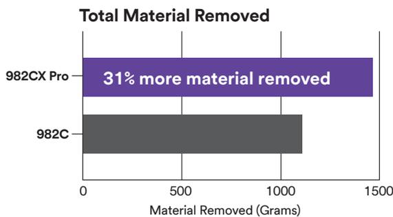
\*Results based on an automated, 11 minute test on 1018 steel using a 3M™ Cubitron™ II Fibre Disc 982CX Pro, 7", grade 36+ and 3M™ Disc Pad Face Plate Ribbed 80514 on a servo motor.
