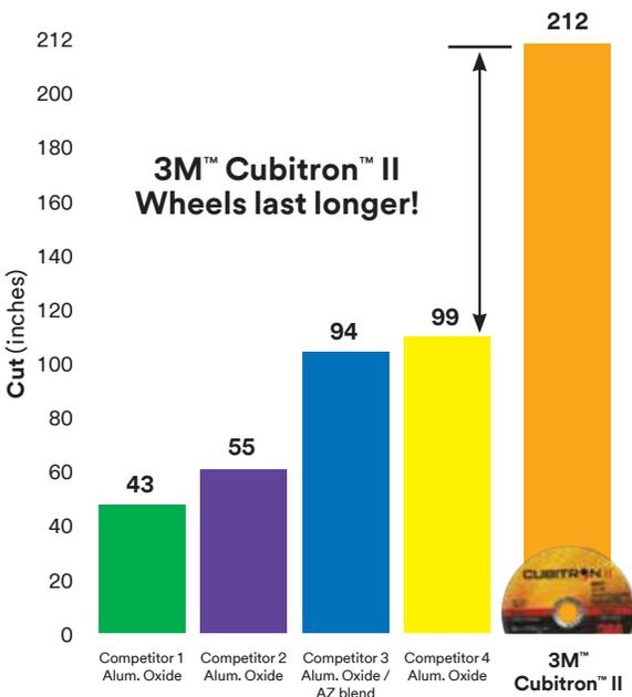
Internal 3M testing on 304L stainless steel sheet (11 gauge) using a 13 amp electric tool.
