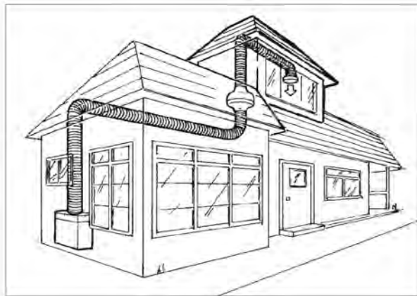
(In-Line Fan) transferring conditioned air to a new room addition
