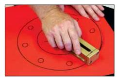
8. With slight downward pressure on cutting block and material, rotate cutter block clockwise to make cut. For thicker or hard to cut materials, make several passes to make cut. Or cut half way through material, turn over and complete cut. On difficult materials (hard, soft, etc.) consider using Easy Cutting Lubricant.
