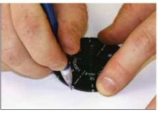
4. Equally space marks around bolt hole locator for the number of bolt holes to be made. Use the number notches on bolt hole locator for reference. For 4 bolt holes, make marks at 1, 4, 7 and 10. For 8 holes make marks at 1, 4, 7, 10 and directly between 2-3, 5-6, 8-9 and 11-12. For 12 holes make marks at 1 through 12. For 24 holes make marks at 1 through 12 and directly between each number.
