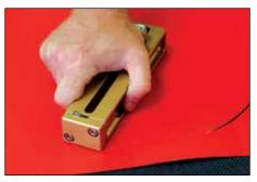
**3.** From gasket material, cut arcs of gasket material with desired OD and ID.
