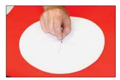
**3.** Place template on gasket material and push disc pin into gasket to make an indentation.
