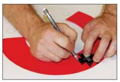
5. Center dovetails on overlapping material and outline with sharp pencil or awl. Cut along outline with knife or scissors. Top and bottom materials will now have mating dovetails. Tape the dovetail joints together for easy handling.
