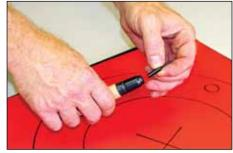
2. Insert center pin into center pin handle. Pierce center of the gasket with the appropriate length center pin for the thickness of material being cut.
