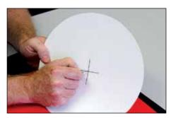
**2.** Push disc pin through center hole from bottom of template.
