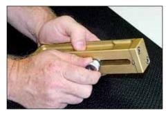
2. Loosen knurled nut and adjust pivot post to desired cutting diameter by matching pivot post indicator line with appropriate dimension of 0"-2" scale. Secure with knurled nut.
