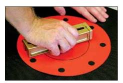
10. Reset cutter block for inside diameter dimension and cut as above.
