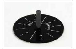
Center bolt hole locator over center point using center pin and press down firmly on its non-slip gripping points. It is essential that bolt hole locator does not move in any way.
