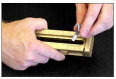
4. Insert thick-headed pivot post without offset pin through cutter block.
