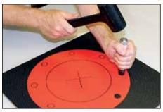
Reset cutter block for bolt holes and cut, or use hole punches to create bolt holes.
