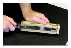
Place extension bar without stud in groove on bottom of cutter block with single, large hole in extension bar toward cutting blade.
