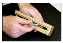
Insert pivot post with offset pin through cutter block, keeping pin toward blade.
