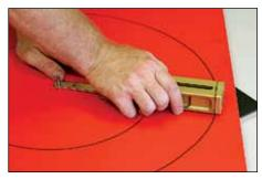
6. With slight downward pressure on cutter block and material, rotate cutter block clockwise to make cut. For thicker or hard to cut materials, make several passes to make cut. Or cut half way through material, turn over and complete cut.
