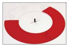
**6.** If gasket is very wide, design two or more side by side dovetails per joint.
