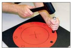
**9.** Reset cutter block for bolt holes and cut, or use hole punches to create bolt holes.
