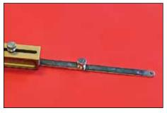
4. To cut gaskets over 25" in diameter, add an additional extension. Use extension bar with stud. Each entension bar adds an additional 12" to capacity of block. Insert stud up through the outer hole on extension already in cutter block. Secure with knurled nut.
