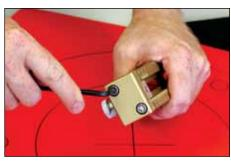
Loosen Allen screws of cutter block and position cutting blade so it protrudes slightly beyond thickness of gasket material. Tighten Allen screws.
