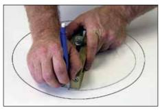
2. From center point of gasket, scribe the bolt hole circle. The gasket cutter can be used as a compass by either holding a pencil against it, or using the cutter blade to create a very shallow cut.
