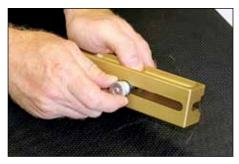
5. Loosen knurled nut and adjust pivot post to desired cutting diameter by matching pivot post indicator line with appropriate dimension of 0"-13" scale. Secure with knurled nut.
