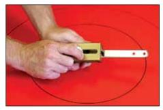
3. Use 0"-13" scale on cutter block. The extension bar adds 12" to capacity of block. To cut a 16" outside diameter gasket, match line through pivot post with the number "4" on scale. Secure with knurled nut.
