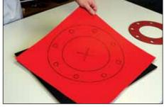
Lay out gasket outer diameter (OD), inner diameter (ID) and bolt holes on template or gasket material. See section 'Using the Bolt Hole Locator'. Ensure the OD of gasket fits the material. If this is not the case, see section 'Using the Dove Tail Designer'.
