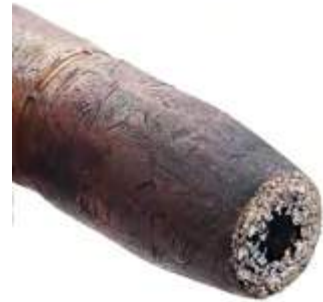
Nozzle fully clogged (not using E-WELD Nozzle)
