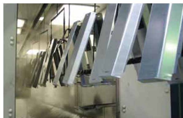
Alkaline cleaner being sprayed on parts.
