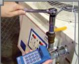
...into a highly accurate digital torque tool.
