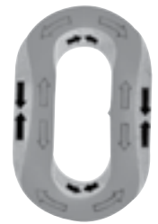
Figure 1 : Pattern of tensile and compression stress shown by a link under load.
