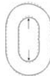
Figure 4 : Changes in link shape that take place under axial tension loading.
