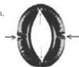
Figure 5 : The tube "under load" shows wrinkles in the areas of compression.
