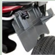
Side Baffle For directional control of spread
