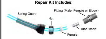
Traditional Nylon Repair Kit contains all items necessary for repairing one tube end. Kit includes fitting, tube insert, ferrule, nut and zinc-coated spring guard.
