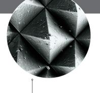
Trizact grain featuring microreplicated three-dimensional abrasive structures for the finest finishes.
