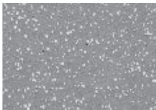
Unique HSS-E-PM material used for SHARK TAPS (note the evenly dispersed grain structure)
