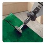
DIAMOND WHEEL -**545** Great for cutting, sawing and carving of hard materials such as marble, concrete, brick, porcelain, ceramics. hard epoxy, soft and hard wood. Mandrel 402 is included. Thickness .023" (0,6 mm). Do not run in excess of 20,000 RPM.
