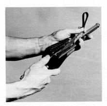
Depress idler arm lever and pull belt toward the contact wheel.
