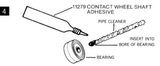
MOISTEN TIP OF PIPE CLEANER WITH CONTACT WHEEL SHAFT ADHESIVE AND APPLY TO ID OF BEARINGS BEFORE INSTALLING PROPER SHAFT.
