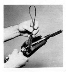
Form a loop in belt keeping the belt splice between fingers as shown in photo above. Slip lower loop of belt under the drive wheel.
