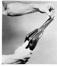
Slip belt over contact wheel. Release idler arm lever. Operate on the contact wheel or on the return side of the belt.
