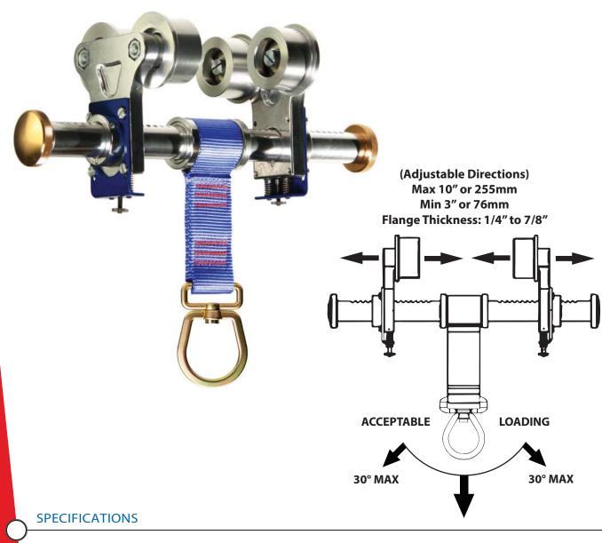
UTS 5,000-lbf / 22kN Max User Weight 310-lbs / 140kg Working Load 1000-lbs / 454kg
