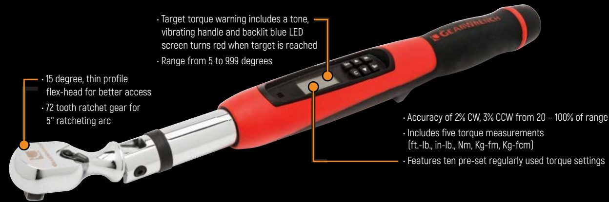
85078 3/8" Drive Electronic Torque Wrench with Angle, 10-100 ft. lbs.
