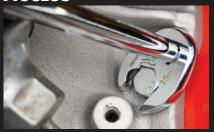
Use with an extension to reach hard to access nuts or when there is not enough clearance to use a ratchet
