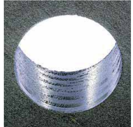
Hole D = 6.35 mm Unidirectional CFRP with optimal machining quality
