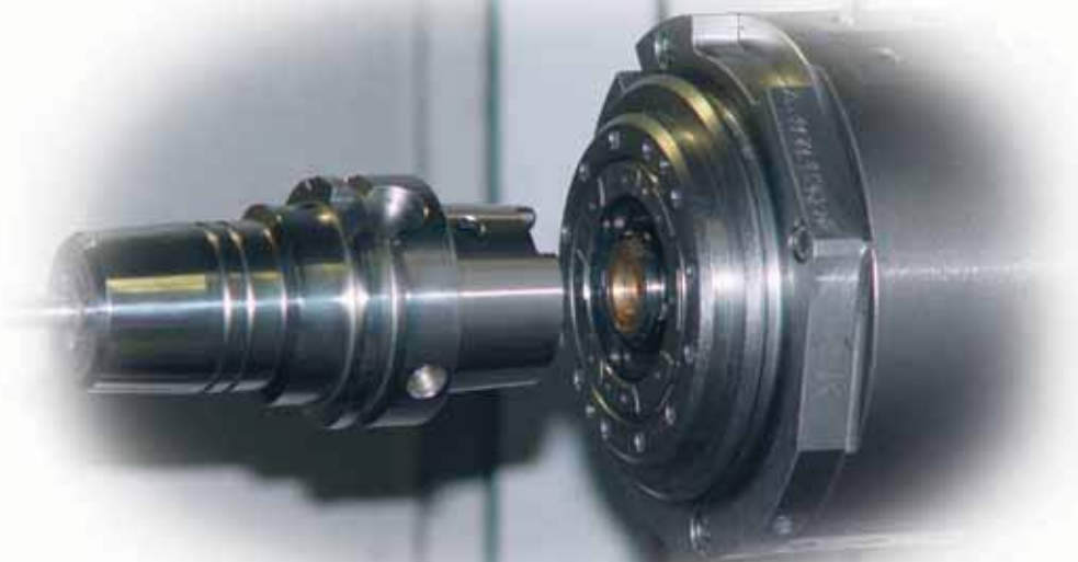
Fig. 1: HSK-A 63 interface, automatic tool change
