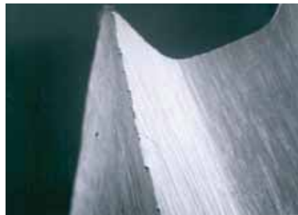
Surface of a conventional fluteless tap
