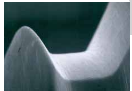
Optimised surface of a Guhring Profile fluteless tap
