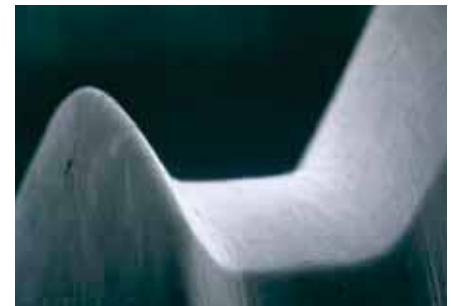
Optimized surface of a Guhring Profile fluteless tap
