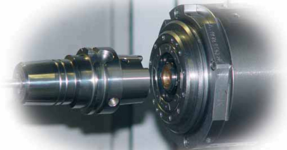
Fig. 1: HSK-A 63 interface, automatic tool change
