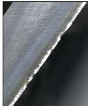
OSG's VGx ® -5: Mild Chipping; Good Wear
