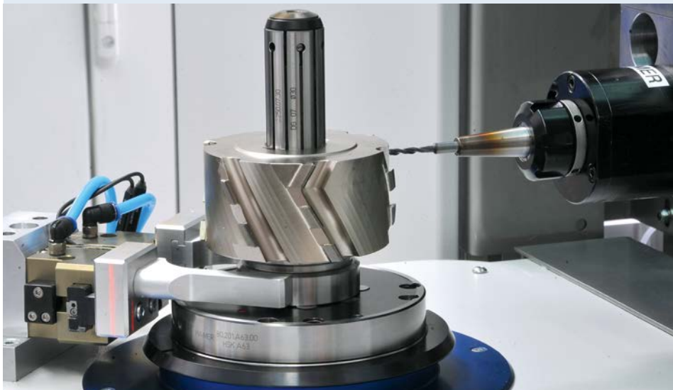
Tools for woodworking Balancing avoids breaking of cutting edges and vibrations and enables the highest accuracy at the edges of the piece of furniture. Thus you raise your productivity and you can realize a higher cutting capacity.
