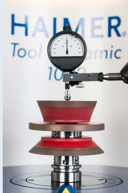
Axial runout check
