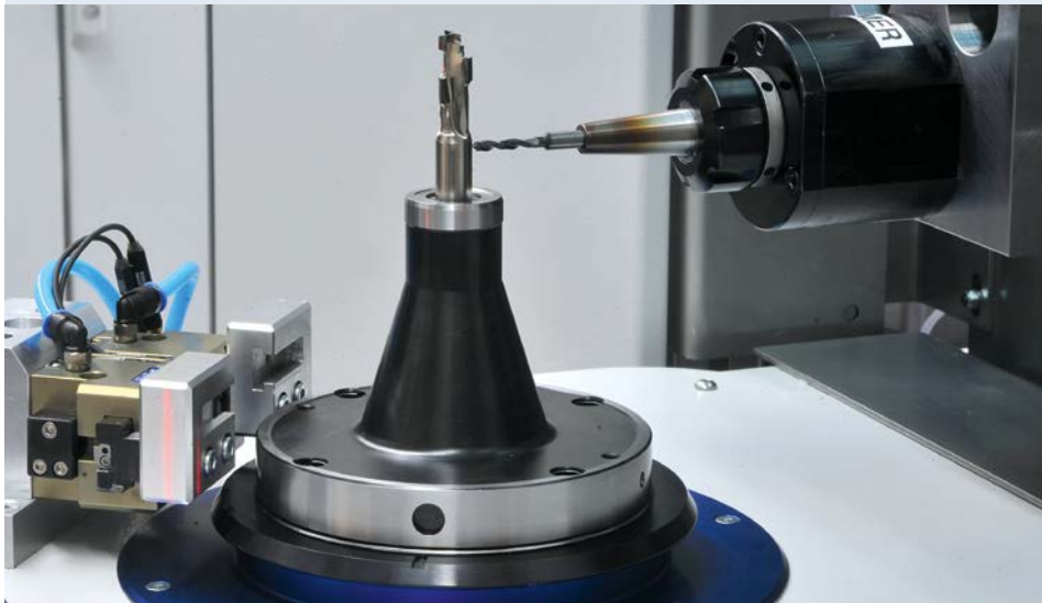
Balancing of tools with a HG balancing adapter for tools with a cylindrical shank
