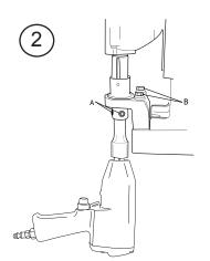
One method is to use an 1/2 drive Impact Gun with a short extension (refer to dia. 2). The extension can be installed into the bottom of the Arbor Body Assembly as a cutter would. Tighten the set-screws (A) and use the Impact Gun in the counter-clockwise direction to remove the Arbor Body.
