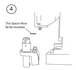
When the Arbor Body Assembly is removed be aware of the Spacer between the Arbor Body Assembly and the Motor Assembly. Refer to the next page to install the 3-Jaw Chuck Assembly.
