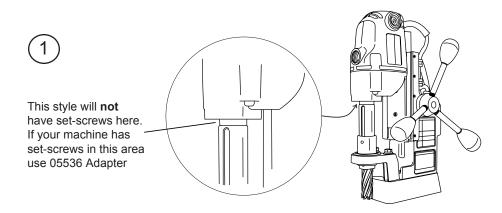
There are 2 methods to remove the Arbor Body Assembly from a threaded style spindle.
