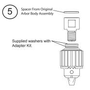
Thread the 3-Jaw Chuck onto the Spindle Adapter keeping the supplied washers centered, until tight. Now thread the complete assembly up onto the bottom of the motor.
