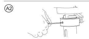
Rotate the Arbor Body so the 5/16-18 X 3/8 set screw inside, aligns with the hole in the Coolant inducer. Insert the 5/32 Hex Wrench and turn the inside set screw 1 full turn counterclock-wise or until loose.
