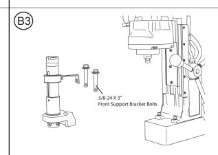
Remove both 3/8-24 X 3" Hex Bolts from the Front Support Bracket using a 9/16 wrench. Now the entire Arbor Body Assembly can be removed.
