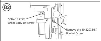
Remove the 10-32 X 5/8" Bracket Screw with a 5/32 Hex Wrench and slide the Brass Coolant Inducer down. Turn the 5/16-18 X 3/8 Set Screw until loose and slide the Arbor Body OFF the Motor Spindle.
