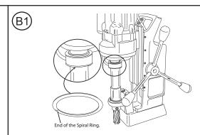
Locate the end of the Spiral Retaining Ring under the Brass Coolant Inducer, and with a pick, pull the end down. Once started, pull the rest of the Retaining Ring down the Arbor Body.
