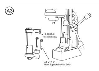
Locate and remove the 10-32 X 5/8" Bracket Screw with a 5/32 Hex Wrench. Remove both 3/8-24 X 3" Hex Bolts from the Front Support Bracket using a 9/16 wrench. Now the entire Arbor Body Assembly can be removed.
