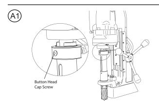
Locate and remove the 1/4-28 X 1/4 Button Head Cap Screw from the Coolant Inducer with a 5/32 Hex Wrench.
