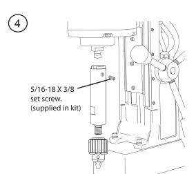
Installation of the Chuck and Adapter is the same on either system covered by the first page. Slide the Spindle Adapter (07301) up onto the Motor Spindle verifying the Spindle sits down in the slot of the Adapter. Install and tighten the 5/16-18 X 3/8 Set Screw (40256), supplied in the kit. Thread the Chuck onto the bottom of the Adapter until hand tight.
