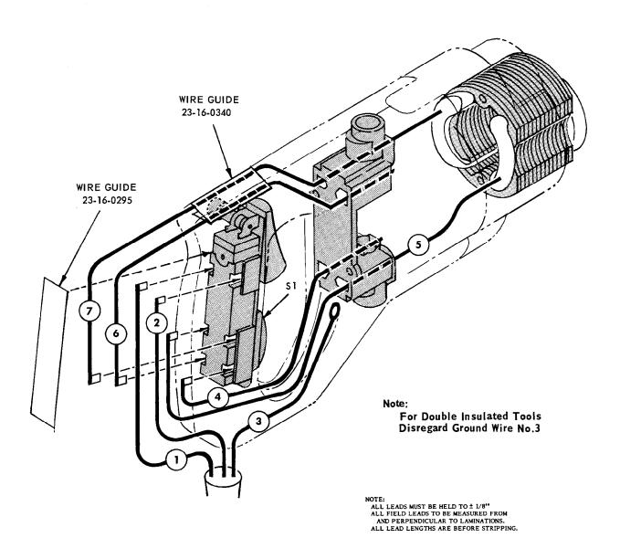
WHERE TERMINAL AND CONNECTOR COMBINATIONS ARE SPECIFIED, SEE ELECTRICAL PARTS CHART FOR PART NO. AND QUANTITY AND DRAWING FOR ACTUAL HOOK-UP
