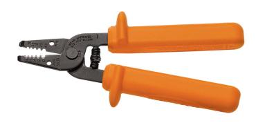
This compact, lightweight wire-stripping, cutting tool cuts, strips, loops and gauges 10-18 AWG solid wire. Dual layer orange-over-white insulation protects against electric shock. Exceeds IEC 60900 and ASTM F1505 standards for insulated tools, and are clearly marked with the official 1000-volt rating symbol. Hardened spring steel with precision-ground stripping holes for easy removal of insulation.
