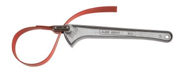
The Klein Tools 12-Inch Grip-It Strap Wrench is completely adjustable for tight-quarters tasks on polished, PVC and glass pipes, fittings, filters, conduit and shafts. The strap is urethane-coated to resist scratching or damaging surfaces and is attached to a lightweight I-beam handle. Also available in 6-Inch and 18-Inch lengths (Cat. No. S6H and S18H).
