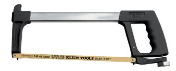
This versatile hack saw blade has three teeth sizes and the ability to quickly convert the blade to 90- or 45-degrees for standard or flush-cut applications. The Pivot-lock adjusts blade tension for straighter cuts and longer blade life. It also features a set screw which allows for storage of extra blades and secutres blade for "jab" sawing.
