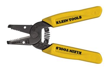
The Klein Tools Wire Stripper/Cutter is a compact and lightweight tool for your stripping and cutting needs. Made from hardened steel for strength, it cuts, strips, loops and bends solid wire. The narrow nose reaches into confined spaces.
