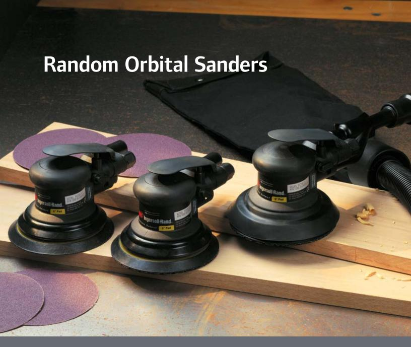
Cyclone random orbital sanders deliver unsurpassed reliability, with moisture-resistant composite rotors, fully machined counterweights, and large counterweight bearings. They are lube-free when used with conventional air systems. Their highperformance air motors ensure high speed under load, and the finest in swirl-free finishes.
