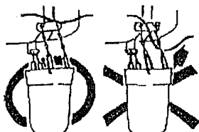
Fig.17 Cables should not pass inside of hangers
