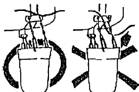
Fig.17 Cables should not pass inside of hangers
