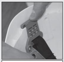
**STEP 4:** Repeat for all four clips making sure they are firmly pressed in place.
