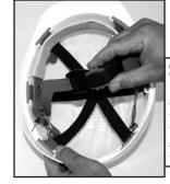
**STEP 9:** Pick up the wheel ratchet labelled 5 in step 1. Locate the two holes at the rear of the head piece and push the two pins on the wheel ratchet through the holes. Repeat on the other side to attach the wheel ratchet and complete the harness
