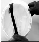
**STEP 2:** Take strap 1 and place it in the front left clip slot. Make sure the tail is facing away from the peak towards the back of the helmet. Push downwards firmly until you hear a click.
