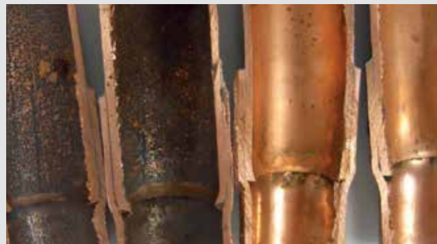
Without nitrogen purge
