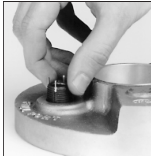
Easy installation: drill out old threads, countersink, tap, screw inserts in place.
