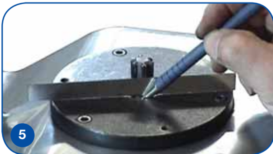
5 You must maintain a specified height between the shoulder and base plate to be within 0.050 and 0.100 in. for proper operation.
