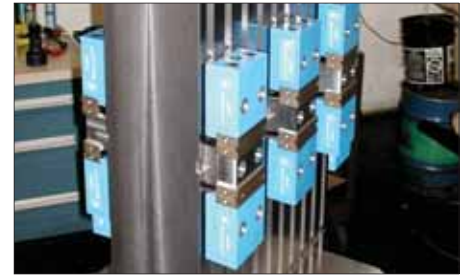
Solution: Two-sided tombstone with six MoveLock clamping stations handle wide range of part sizes.
