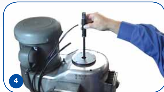
4 Slide washer in to position and install drawbar in the top of the mill.
