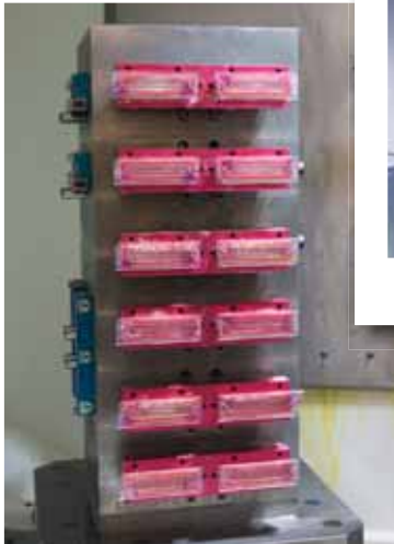
DoveLock jaws used for glass machining
