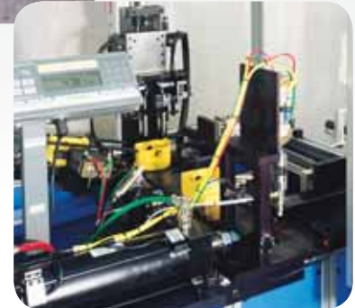
In-Line Fully Automated Gage Fixture
