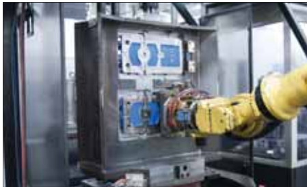
Solution: Window fixture for 2 sided machining enhances automated FMS line.
