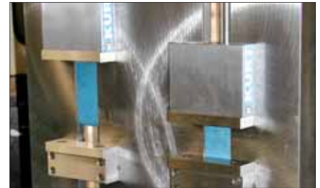
Solution: D100 movable and stationary jaws integrated onto a tower.
