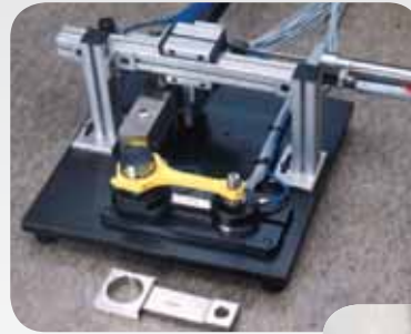
Bench-top, post-process gaging fixtures configured around any part
