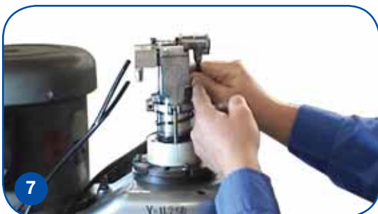
7 Properly identify and install air lines to appropriate locations.
