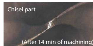
Good without fracture
