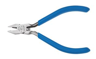
These 4-Inch Klein Tools Midget Electronics Diagonal Cutting Pliers have a semi-flush design to cut nickel ribbon wire. The nose tip is 1/32-Inch and the tip cutting knife is 3/16-Inch for precision in tight areas. Finally the pliers are forged from US steel and have induction hardened cutting knives and a hotriveted joint for a long lasting smooth action.
