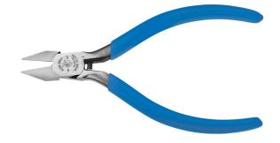
These Klein Tools 5-Inch, Electronics Pliers have a narrow jaw and hinge with a sharp pointed nose for precision in tight areas. These short jaw pliers have beveled standard cutting edges for perfectly flush cuts. They are made of US-made steel and are induction hardened with a spring assisted hot-riveted joint for a smooth action and long lasting durability.
